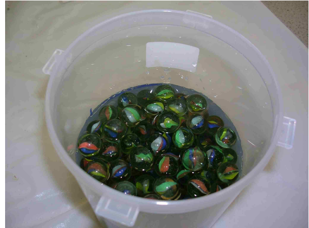
Measuring the ‘porosity’ of a container of glass marbles
