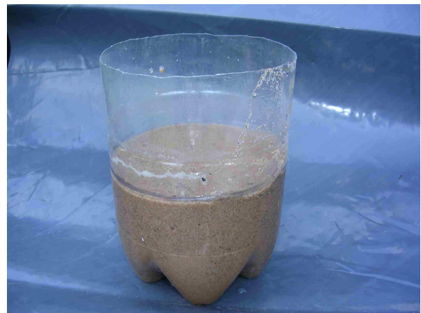
Measuring the porosity of a container of loose sand (Photos: P. Kennett)
